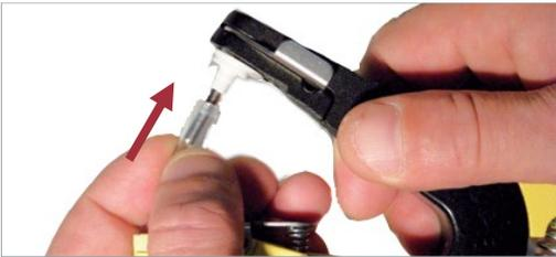
Attach the two parts together by applying sufficient pressure until the plastic tube “clicks” into place on the base of the stainless steel tube part. Make sure both pieces (needle and tube) are inseparably fixed to each other.
