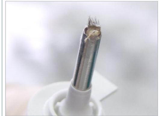
If the pink cross shaped piston is still visible after sampling, the needle is empty.
